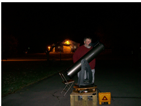
ROUND TABLE PLATFORM. Mark Coody demonstrates the Round Table Platforms equatorial tracking platform. Adds equatorial capability to Dobsonian mount.
